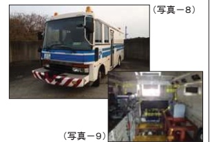
※動的たわみ計測装置(MWD: Moving Wheel Deflectometer)
